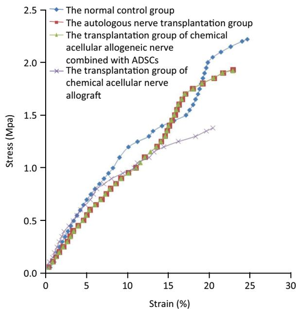
**Figure 2** - Tensile stress-strain curves of the sciatic nerves from different groups.
